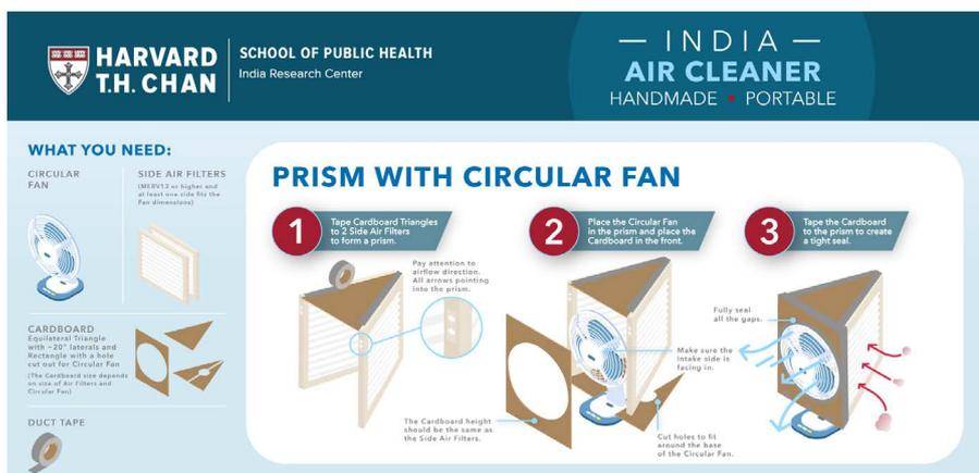
Reduce your indoor exposure to COVID-19. Learn how to make a portable do-it-yourself prism air cleaner with a circular fan to remove contaminants such as viruses from the air.
